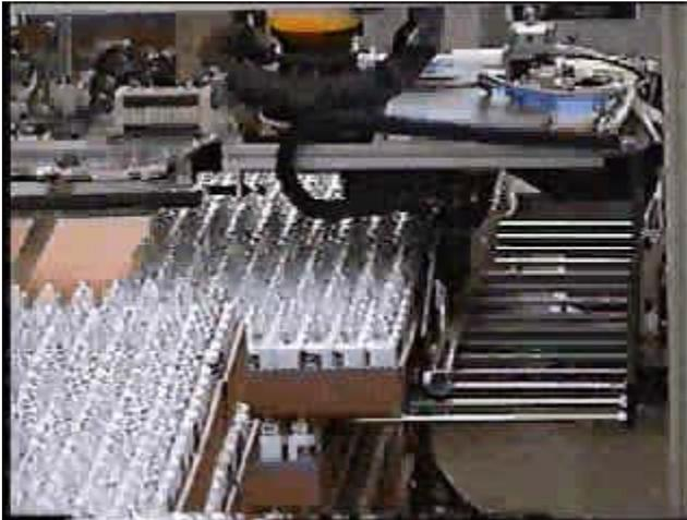
Using a **vacuum tool** is the least expensive method available. Vacuum cups come in a variety of styles and sizes and work best with products in non-porous bags with flat surfaces (such as plastic). This method also works best with products that are tightly packed. Tightly packed products, as opposed to fluid product, will allow the bag to maintain its shape which in turn allows the vacuum to maintain its contact with
