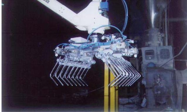
gripper approach. While this method has the added advantage of holding the bag more securely while in motion than the clam shell of vacuum methods it does require a specially designed conveyor to allow its “fingers” to pick and it requires more room in which to operate.
